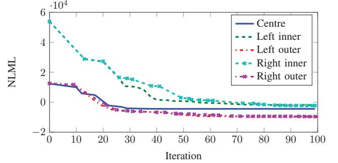
Fig. 4: Negative log-marginal likelihood of the GPR models for the longitudinal C.G. during the offline training operation.
