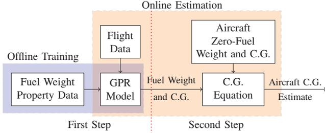
Fig. 1: Block diagram of the proposed aircraft C.G. estimation method using GP regression models.
