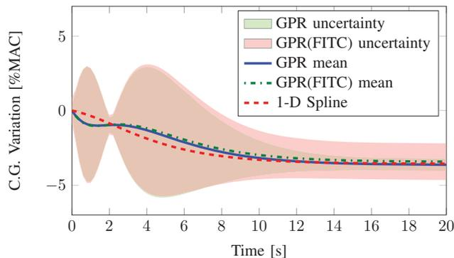
Fig. 5: Estimate of the aircraft longitudinal C.G. variation during level deceleration flight.
