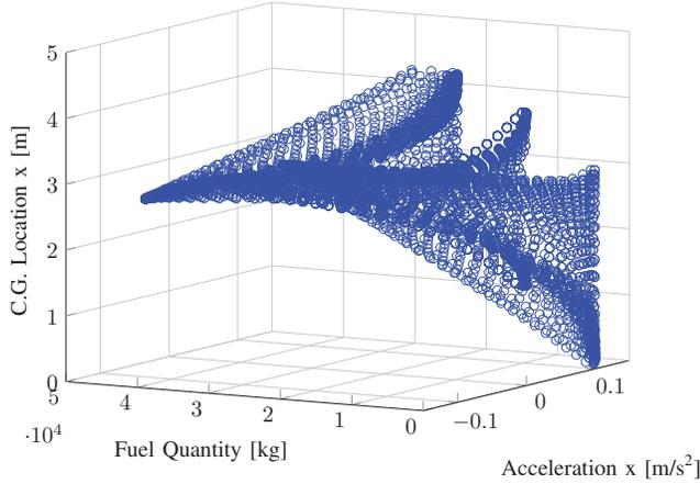
Fig. 3: Scatter plot the the data points in the fuel weight property data of the centre tank.
