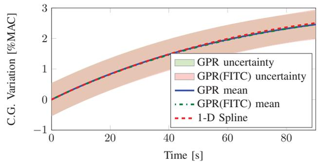
Fig. 6: Estimate of the aircraft longitudinal C.G. variation during cruise flight.
