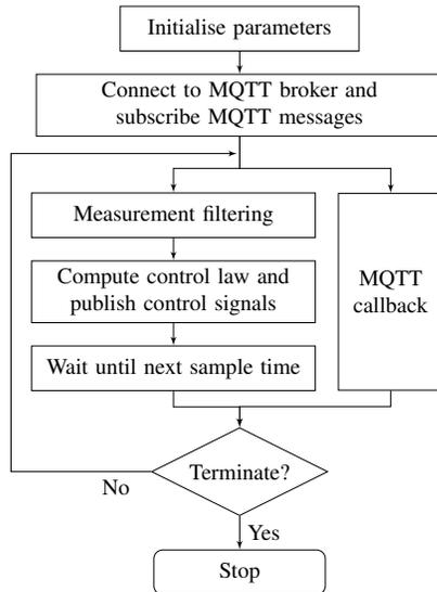
Fig. 8: Flow chart of the controller program of the server software.
