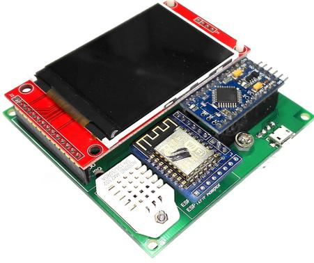
Fig. 4: The finished sensor unit hardware.
