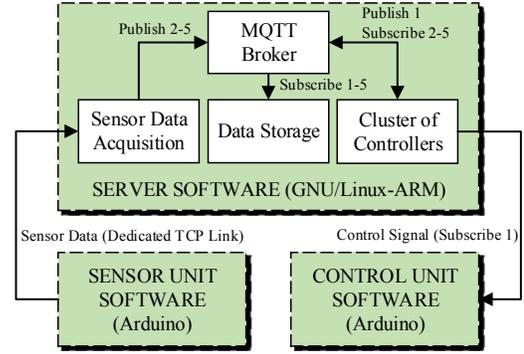
Fig. 7: Software structure of the indoor air quality monitoring and control system.
