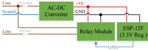
Fig. 5: Interconnections among modules of the control unit hardware.
