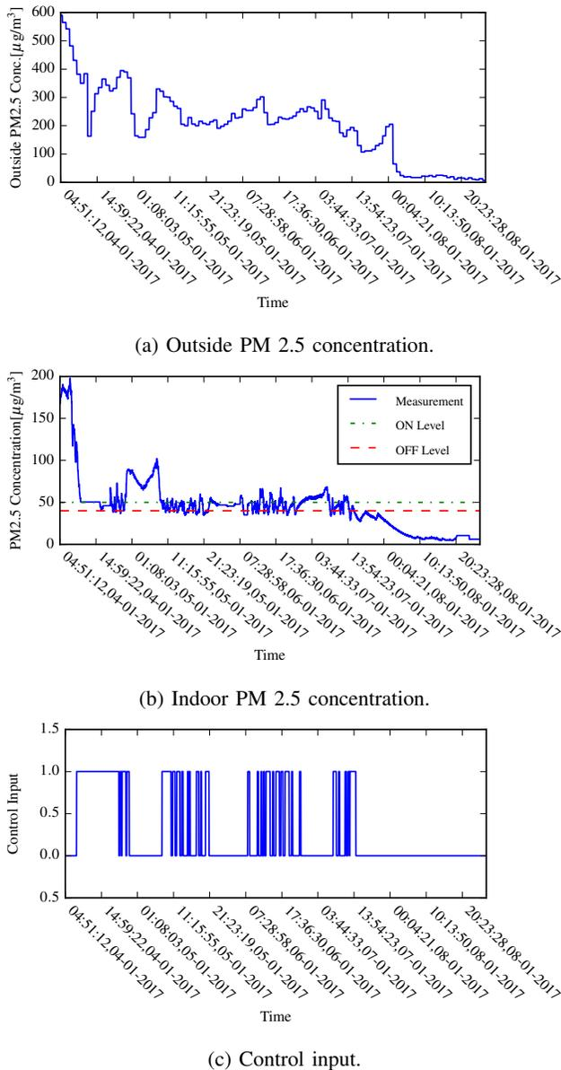
Fig. 11: PM<sub>2.5</sub> concentrations and the corresponding control input in the second experiment.
