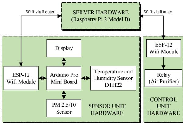
Fig. 1: Hardware structure of the indoor air quality monitoring and control system.
