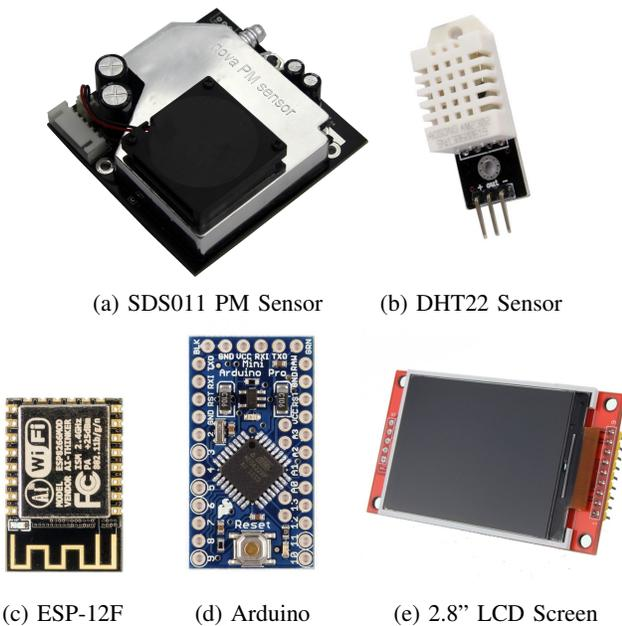
Fig. 2: Individual modules of the sensor unit hardware.
