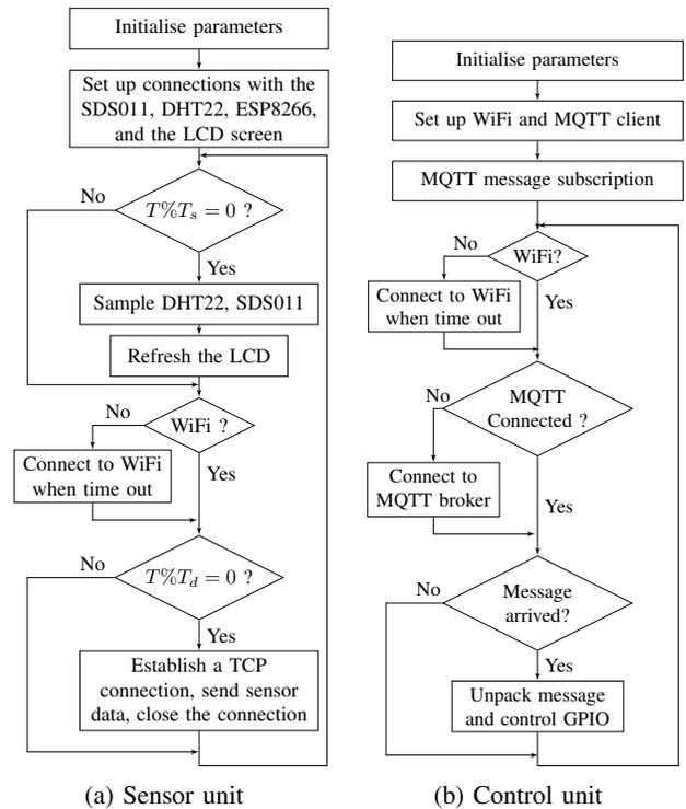
Fig. 9: Flow charts of the sensor and control units software.
