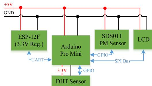
Fig. 3: Interconnections among modules of the sensor unit hardware.
