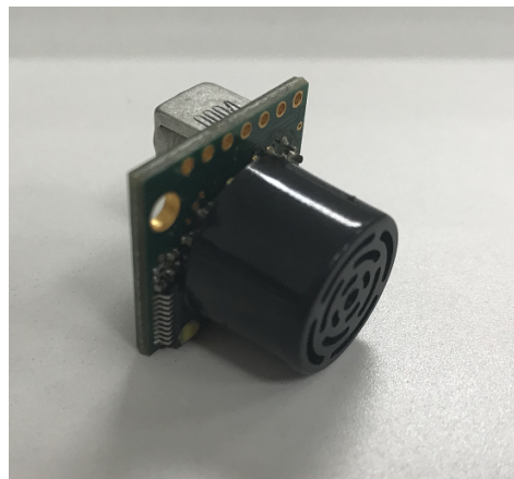
Figure 3. The MB1222 I2CXL-MaxSonar-EZ2 sonar range finder.
